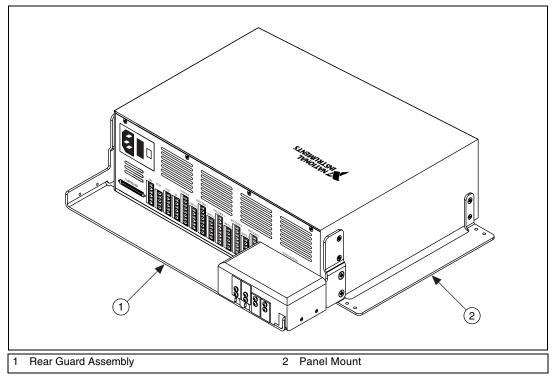
Figure 24. MID-7654/7652 with the Panel Mount Kit Installed
